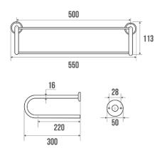
Chrome and nickel-plated brass tube. Polyamide flanges and chrome-plated brass cover plates. Concealed fixings.
