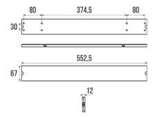
Fixing rail fitted with an anodised aluminium cover, with 2 white resin bolts. The cover can be replaced with a straight grab bar 552 mm or a backrest + 1 armrest or a backrest + 1 hinged bar for shower seat and can thus be used to convert a "Classic" shower into an ergonomical "Comfort" shower.
