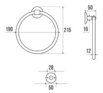
Chrome and nickel-plated brass tube,  $\varnothing$  12 and 16 mm. Polyamide flanges and chrome-plated brass cover plates. Concealed fixings.
