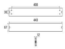
Fixing rail fitted with an anodised aluminium cover, with 2 anthracite resin screws. The cover can be replaced with a straight grab bar of 443 mm or a backrest for shower seat and can thus be used to convert a "Classic" shower into an ergonomical "Comfort" shower.
