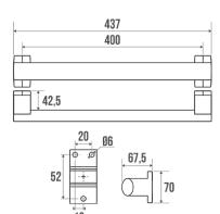
White aluminium tube  $\varnothing$  30 mm, synthetic resin wall fixings and blue synthetic resin cover plates (RAL 1023),  $\varnothing$  66 mm.
