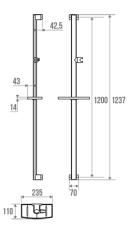
Elliptical anthracite grey epoxy-coated aluminium tube 38 x 25 mm. Anthracite grey synthetic resin cover plates.
