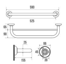
2 fixed arms. Concealed fixings. White synthetic resin flanges and cover plates. Steel tube Ø 25 mm.
