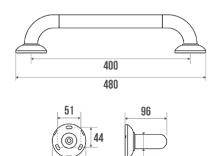
Composite material: White synthetic resin + aluminium profile. Tube  $\varnothing$  33 mm. White flange border and central body. Concealed fixings.
