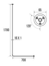
Tube Ø 16 x 1 mm. Can be cut to size. 2 conical tightening wall flange.
