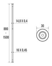
Tube Ø 16 x 0,5 mm. Supplied with flanges, screws and wall plugs. Cannot be shortened.
