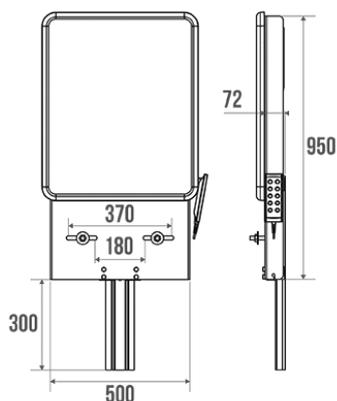
Adjustable height with electrical assistance, with remote control, up to 300 mm.
