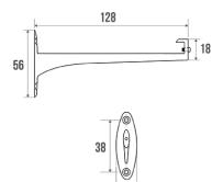
With front screw. For shelves 120 mm deep and maximum 8.5 mm thick. Per pair.
